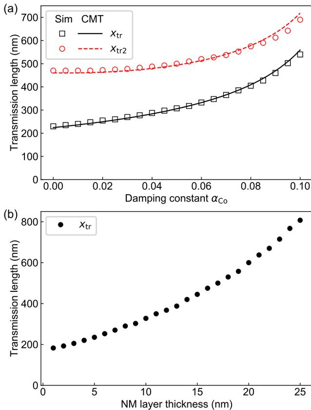
Fig. 4. Transmission length dependence on (a) the damping constant in the Co layer in the Py(3)/NM(5)/Co(2)/Pt multilayer with the damping in the Py  $\alpha_{Py} = 0.005$  and (b) the thickness of NM layer in the Py(3)/NM(x)/Co(2)/Pt multilayer. The source of the SW of 15.2 GHz is located in the Py layer. In (a), the simulations (Sim) results were compared with the Eqs. (10) and (11) from the coupled-mode theory (CMT). In (b), we present the simulations results for  $x_{tr}$  only.
