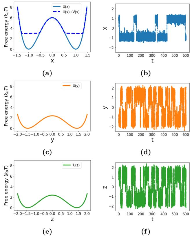
**FIG. 1:** Free energy profile along each degree of freedom of the model system ((a), (c) and (e) respectively) and the corresponding trajectories from Langevin dynamics ((b), ((d) and (f) respectively). In (b) the sum of underlying and bias potentials are indicated with a dashed line.
