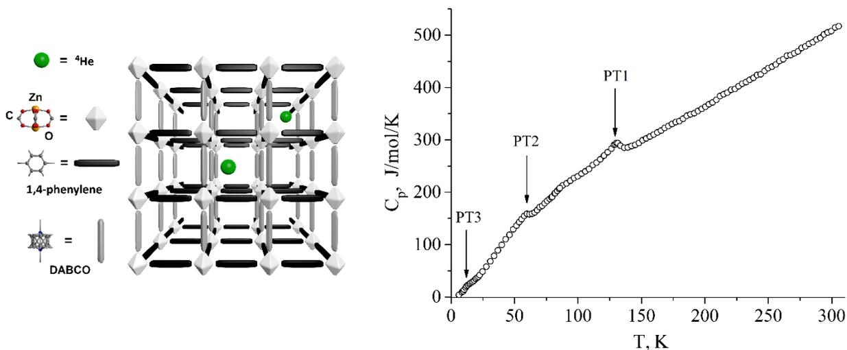
**Fig. 1** Schematic structure of  $\text{Zn}_2(\text{BDC})_2(\text{DABCO})$  whose framework is characterized by a substantial volume of free space (more than 60% of the framework volume). Temperature dependence of heat capacity ( $C_p$ ).
