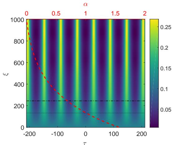
FIG. 7. Color-map of the space-time evolution of steepness  $kU$ , with  $U$  the solution of Eq. (2), over an uneven bottom with linear slope.  $\xi$  and  $\tau$  are in units of m and  $\text{m}^{\frac{1}{2}}$ , respectively, as discussed in the text. The red dashed line shows the variation of  $\alpha$  as a function of  $\xi$  and is mapped on the additional abscissa on the top. The two horizontal black lines (dotted and dashed-dotted) correspond to their counterpart in Fig. 6.
