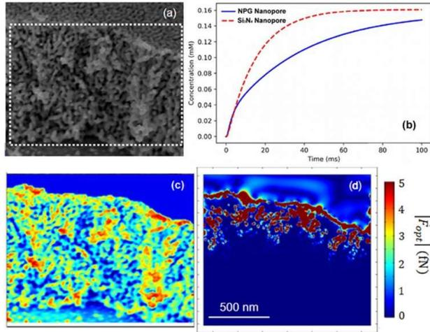
**Figure 3:** (a) SEM image of a cross section of the experimental NPG film (b) The average concentration of the molecules going through the pore against time. (c) The SEM image imported in the numerical FEM model (d) Norm of the optical forces theoretically computed across the cross section of the NPG at  $\lambda = 785$  nm.
