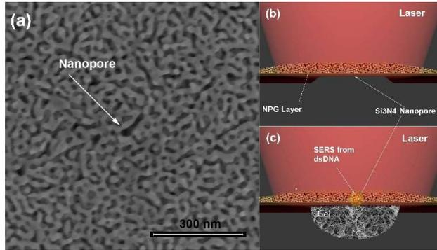
**Figure 1:** (a-c) SEM micrograph of the investigated sample and schematic layout of the structures.
