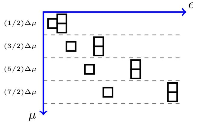
FIG. 2. Schematic of the discrete restacking problem for a spatial region divided between an area with constant field  $B_0$  and an area with constant field  $B_1 = 2B_0$ . Dashed lines separate different values of  $\mu$ . For each value of  $\mu$ , the single box occupies the phase space on the low-field side and the pair of boxes occupy the phase space on the high-field side.
