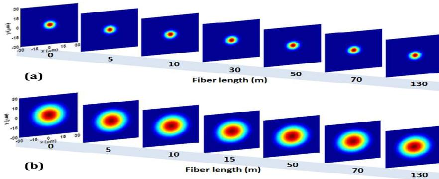
**Fig.6.** Spatial beam evolution in GRIN-F (a) and STEP-F (b) where the most initial energy is coupled in the  $LP_{01}$  mode.
