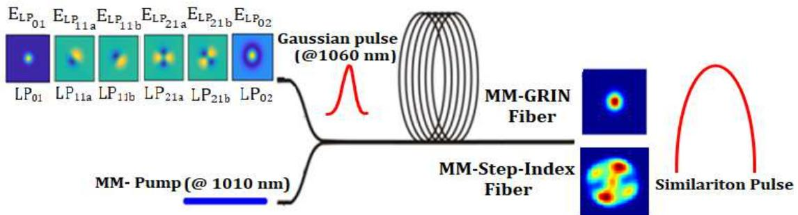
**Fig.1.** Simulation set-up for spatiotemporal evolutions of similariton pulses in MM-Fibers with Raman amplification.
