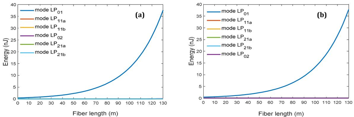
**Fig.3.** Pulse energy evolutions of all the modes in the GRIN-F (a) and the STEP-F (b) where the most initial energy is coupled in the  $LP_{01}$  mode.
