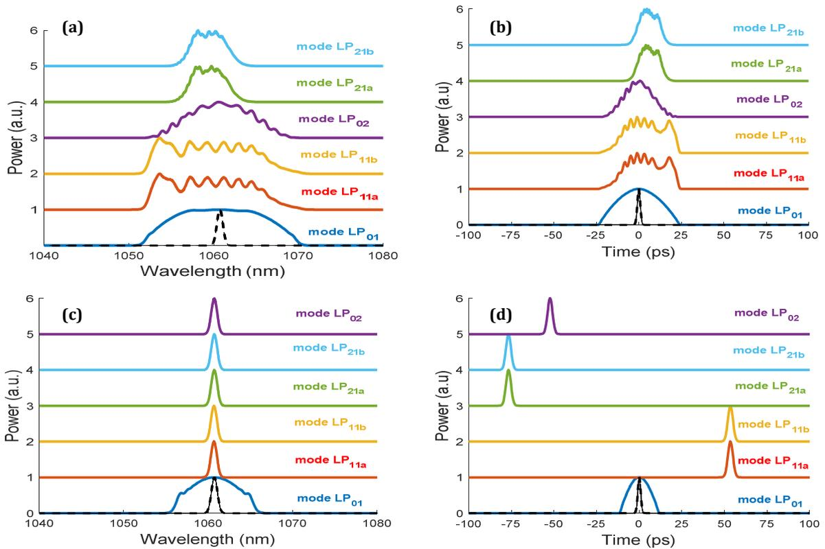
**Fig.2.** Spectral and temporal forms for 130m of pulse propagation for all the modes in the GRIN-F (a and b) and the STEP-F (c and d). Dashed line represents the initial pulse form.
