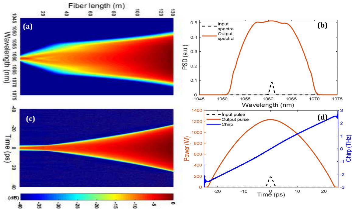
**Fig.4.** The spectral and the temporal similariton evolutions (a and c) and output forms (b and d) of the LP<sub>01</sub> mode in GRIN-F.
