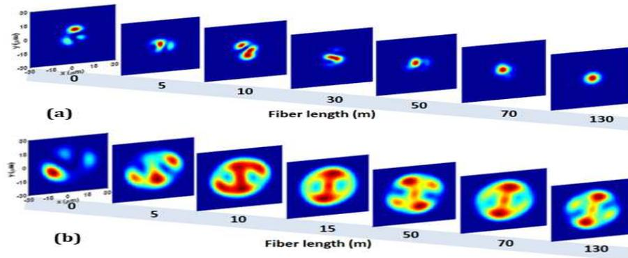
**Fig.7.** Spatial beam evolution in GRIN-F (a) and STEP-F (b) where the initial energy is equally distributed among all the modes.
