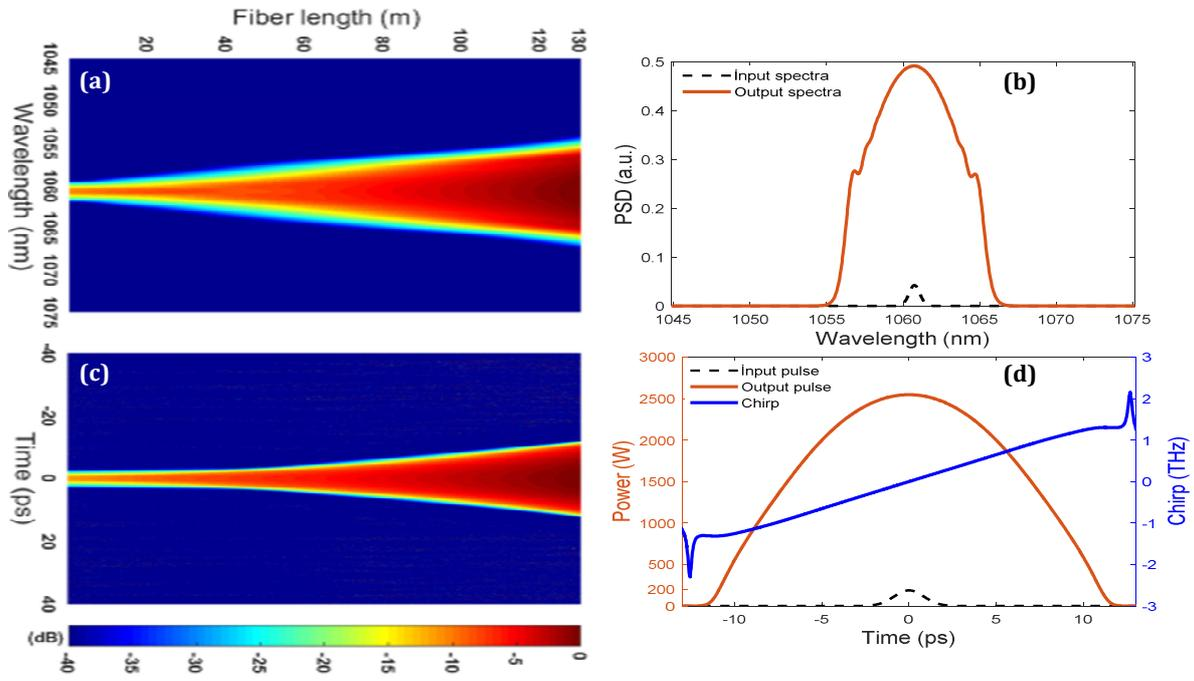
**Fig.5.** The spectral and the temporal similariton evolutions (a and c) and output forms (b and d) of the  $LP_{01}$  mode in STEP-F.
