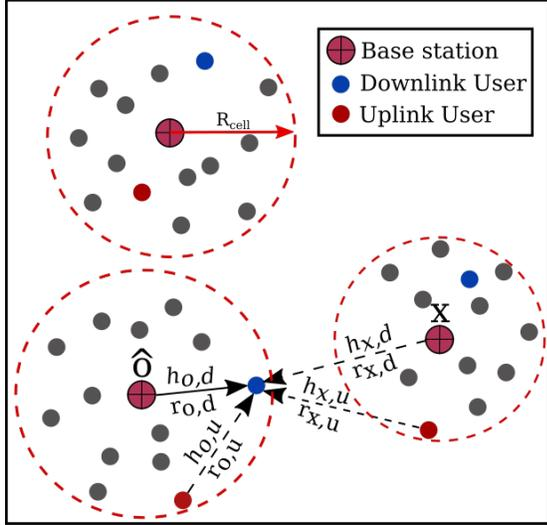
Fig. 1: A snapshot of the network. The UEs are clusters of radius  $R_c$  around the parent BS. A downlink UE of cell will be served by the parent BS of the cell; uplink UE(s) allocated in the same resources are marked in red.
