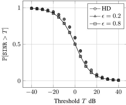
Fig. 2: Coverage probability of a typical downlink user in HD and FD for various different power control factor  $\epsilon$  with fixed  $P_0 = -64 \text{ dBm}$ ,  $P_d = 40 \text{ dBm}$  and Inter-BS distance 400m. Simulations are marked by  $\oplus$ .
