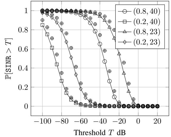
Fig. 3: Coverage probability of a typical uplink user for various configuration  $\epsilon$  and  $P_d$ ,  $(\epsilon, P_d)$  with  $P_0 = -64 \text{ dBm}$  and inter-BS distance 400 m. Simulations are marked by  $\oplus$ .
