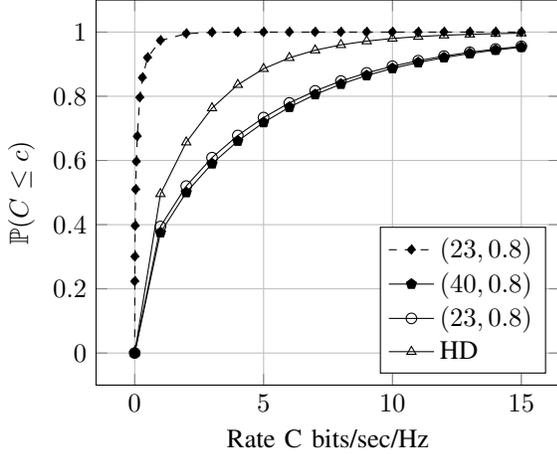
Fig. 5: Rate CDF of a typical uplink/downlink user in FD with uplink power control for various configuration  $P_d$  and  $\epsilon$ ,  $(P_d, \epsilon)$  with  $P_0 = -64$  dBm and inter-BS distance 400m. Uplink coverage is shown by dashed line.
