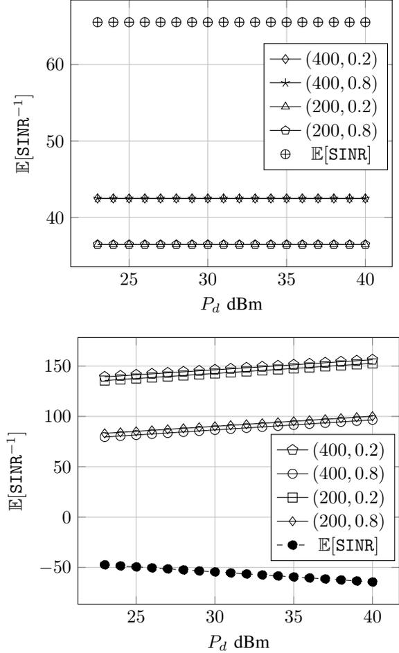
Fig. 4: Expectation of  $\text{SINR}^{-1}$  of a typical downlink (above)/ uplink (below) user in FD system with uplink power control against different values of downlink power  $P_d$ , for various  $\lambda$  (depending on  $R_c$ ) and  $\epsilon$ ,  $(R_c, \epsilon)$  with  $P_0 = -64$  dBm.  $\mathbb{E}[\text{SINR}]$  is obtained using simulations.
