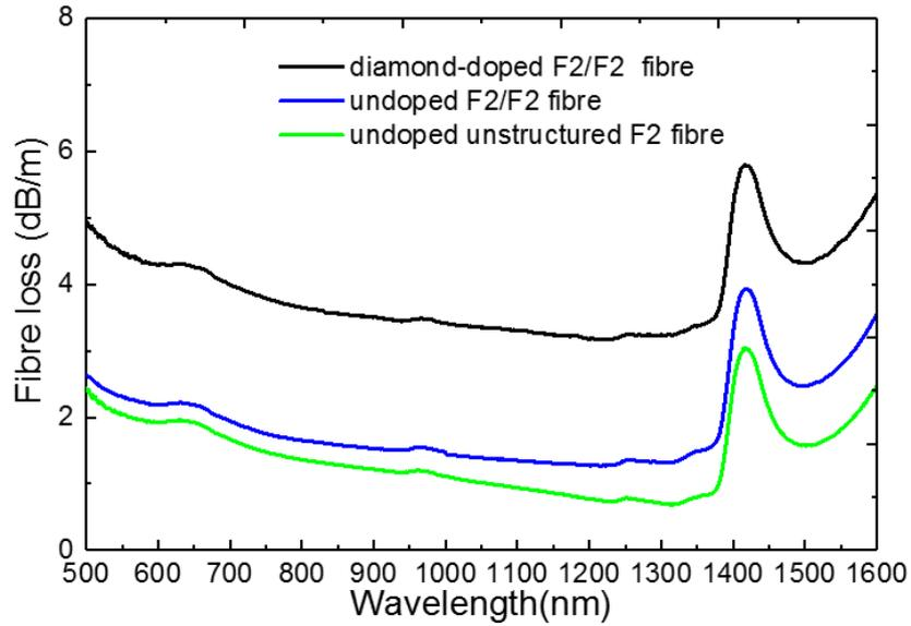
**Figure 2.** Propagation loss of diamond-doped F2/F2 fiber (black curve), undoped F2/F2 fiber (blue curve), and unstructured undoped F2 fiber (green curve) in wavelength range of 500-1600 nm. The relatively higher loss of diamond-doped F2/F2 fiber is mainly due to scatterings induced by the diamond particles. Comparison between the two undoped fibers indicates the interface holes have insignificant impacts on the fiber loss.
