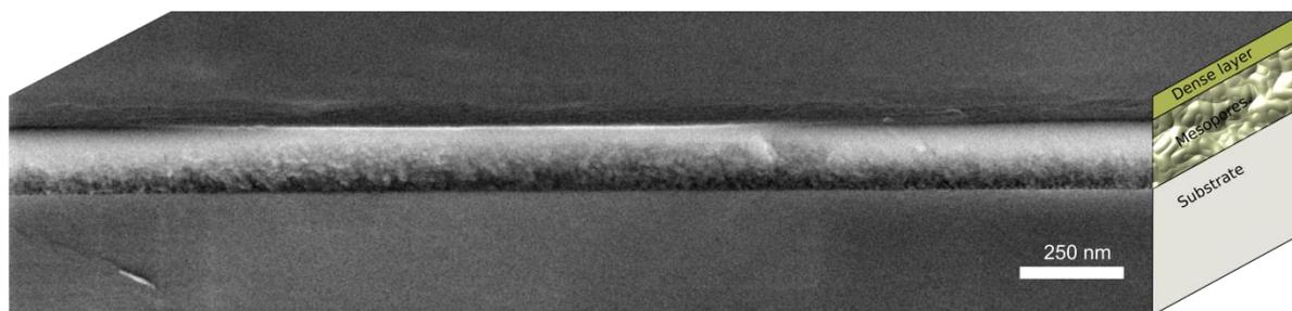
Figure S 1: Large scale scanning electron micrograph of sample A showing the substrate, the mesoporous, and the dense layers. On the right, a sketch of the sample structure is included as a guide to the eye. The interface between the mesoporous layer and the dense SiO<sub>2</sub> layer is much smoother than the top surface of the dense layer. The SEM image was taken before Ni deposition.
