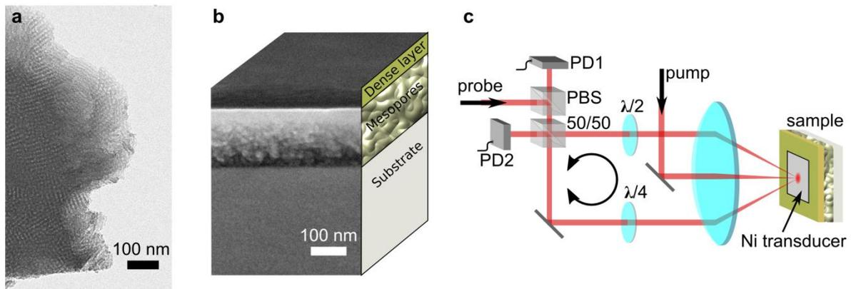
Figure 1: **a** TEM image of  $\text{SiO}_2$  mesoporous film showing the mesopore array. **b** SEM micrograph of sample A showing the substrate, the mesoporous, and the dense layers. On the right, a schematic of the sample is presented as a guide to the eye. **c** Interferometric pump-probe setup. A strong pump pulse excites acoustic phonons through partial absorption in a Ni transducer layer. A probe pulse detects the time-resolved surface displacement using a Sagnac interferometer.[37], [38]
