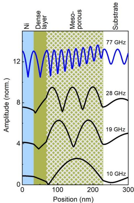
Figure 3: Numerical simulation of the mode-spatial profiles corresponding to the sample C. The curves from bottom to top correspond to 10, 19, 28, and 77 GHz, respectively. The curves have been vertically shifted for clarity. The three lowest-frequency modes show an evident standing wave character in the mesoporous layer.
