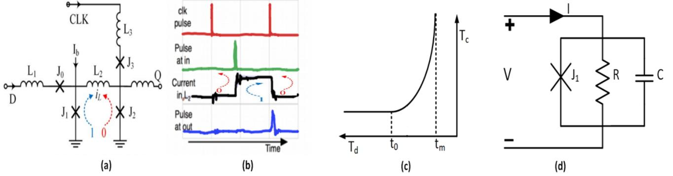
Fig. 1. (a) Schematic of a DFF (b) Simulation result of a DFF in SFQ (c) Illustration of clock-to-Q delay  $T_c$  as a function of the arrival time of the data pulse  $T_d$  relative to the clock. (d) RCSJ model of  $J_1$
