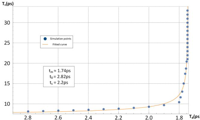
Fig. 3. Clock-to-Q delay ( $T_c$ ) of a DFF as a function of the relative arrival time of the input pulse with respect to the clock ( $T_d$ ). The dotted points indicate simulation results and the overlaid curve is the best fit of our proposed model.
