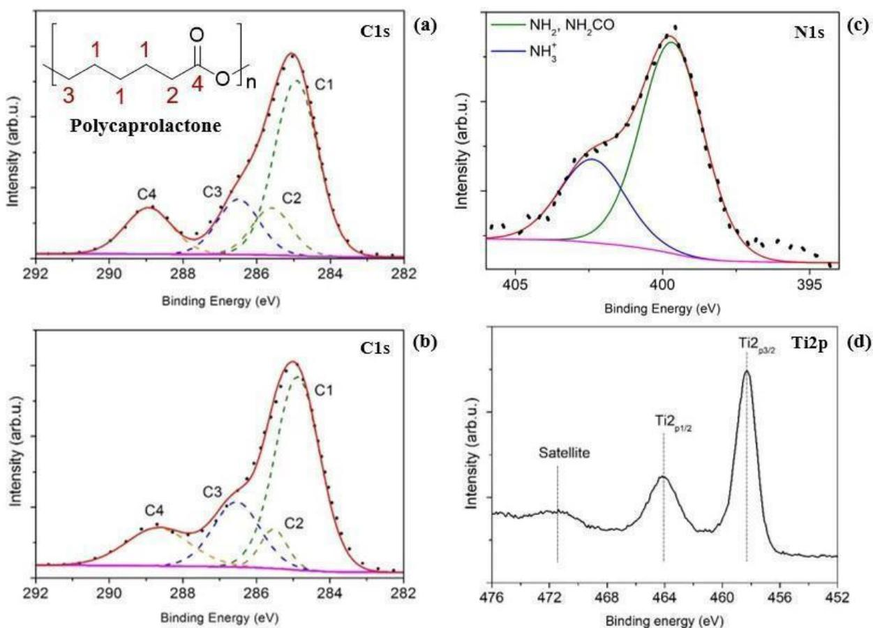
**Fig. 4.** C1s core-level spectra of the control PCL grafts (a); C1s core-level spectra (b), N1s core-level spectra (c) and Ti2p core-level spectra of the PCL grafts immediately after treatment with magnetron DC plasma at 20 W.
