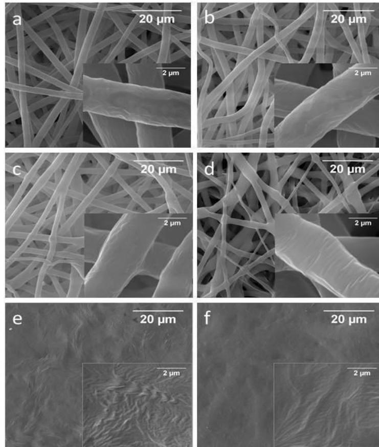
**Fig. 1.** SEM images of the electrospun PCL vascular grafts after plasma treatment at different currents: (a) untreated scaffolds and scaffolds treated at 20 W (b), 45 W(c), 75 W (d), 105 W (e) and 135 W (f).
