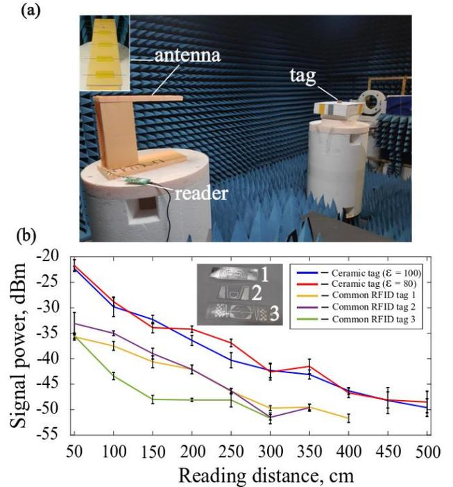
Fig. 5. (a) Photo of the experimental setup in an anechoic chamber – RFID reader with a custom-made Yagi-Uda antenna. (b) Received signal power as the function of the distance between the reader and the tag. Inset shows photograph of the measured commercial tags.
