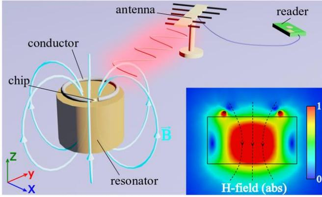
Fig. 1. Operational scheme of a miniature ceramic-based RFID tag. Displacement currents within high-Q resonator are inductively coupled to a metal split ring, functionalized with an RFID chip. Miniaturization and long reading range are ensured by localized modes within high permittivity ceramics. Inset shows the magnetic field amplitude of the fundamental magnetic mode.
