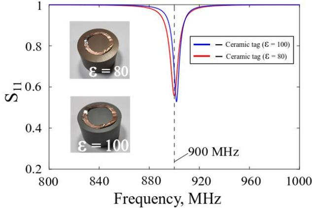
Fig. 3. Numerically calculated  $S_{11}$  spectra of ceramic tags, indicated in legends.  $S_{11}$  parameters were extracted by plugging a port directly to the ring's gap. The impedance of the port is equal to the value, provided by the vendor IC (Impinj Monza 4). Insets shows photographs of the fabricated tags.
