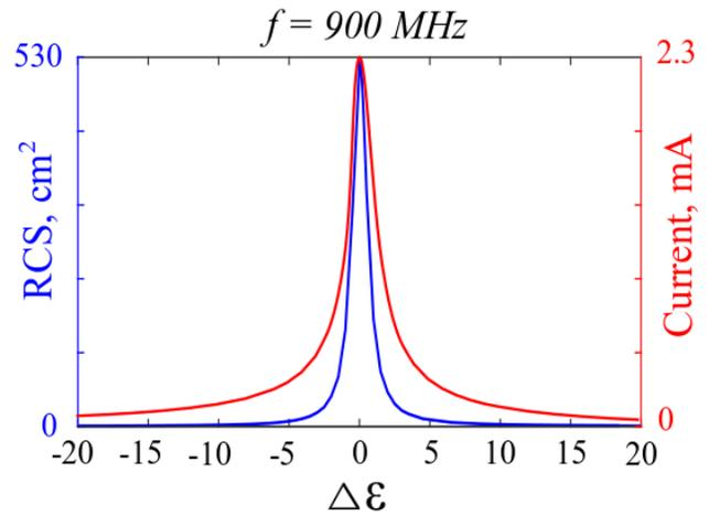
Fig. 4. Ceramic tag parameters as the function of the permittivity detuning. Left scale (blue) – RCS, right scale (red) – the current trough a small resistor. Additional parameters are given in the main text.
