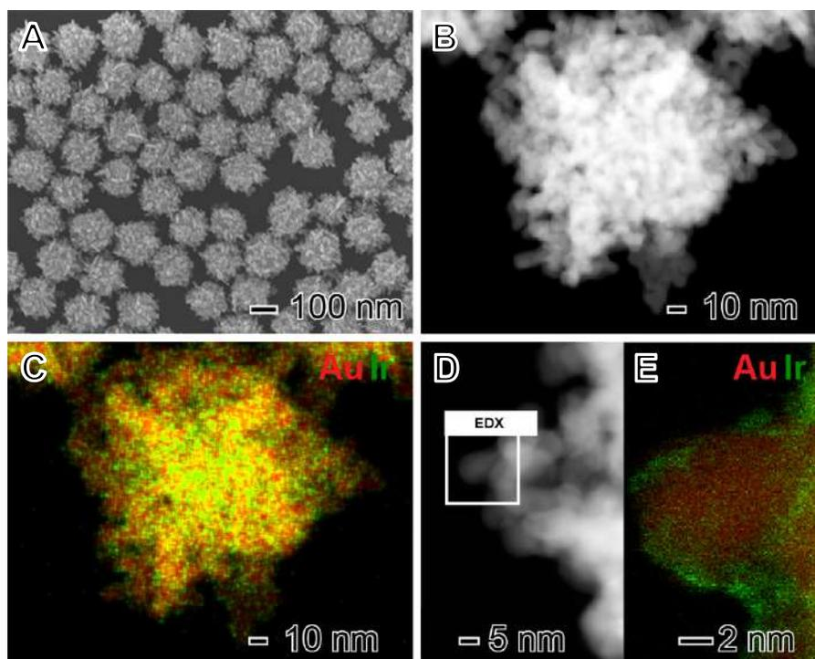
**Figure 2.** SEM (A), HAADF-STEM (C and D) and STEM-EDX (C and E) images for Au-IrO<sub>2</sub> nanodendrites obtained by co-reduction of AuCl<sub>4</sub><sup>-</sup> and IrCl<sub>3</sub>·xH<sub>2</sub>O precursors in a 1:0.25 molar
