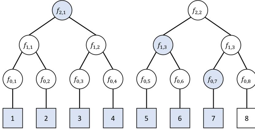
Figure 1: A diagram showing the hierarchical decomposition of the domain  $\{1, \dots, 8\}$  using 14 intervals. The highlighted squares represent the interval  $\{1, \dots, 7\}$  and the highlighted circles show the decomposition of this interval into a union of 3 intervals in the tree.
