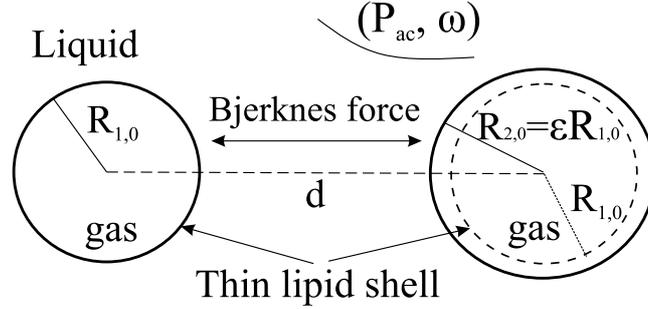
Figure 1: Schematic picture of two interacting contrast agents oscillating in a liquid under the influence of an external pressure field.  $\epsilon$  denotes the ratio between equilibrium radii of two bubbles in static pressure of infinite volume of liquid without any external field, i.e.  $R_{20} = \epsilon R_{10}$ ,  $|\epsilon - 1| \ll 1$ .
