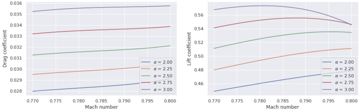
Figure 2: Predictions of  $C_D$  and  $C_L$  from polynomial models
