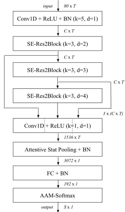
Figure 2: Network topology of the ECAPA-TDNN. We denote  $k$  for kernel size and  $d$  for dilation spacing of the Conv1D layers or SE-Res2Blocks.  $C$  and  $T$  correspond to the channel and temporal dimension of the intermediate feature-maps respectively.  $S$  is the number of training speakers.
