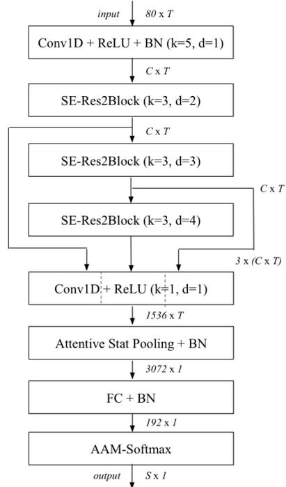
Figure 2: Network topology of the ECAPA-TDNN. We denote  $k$  for kernel size and  $d$  for dilation spacing of the Conv1D layers or SE-Res2Blocks.  $C$  and  $T$  correspond to the channel and temporal dimension of the intermediate feature-maps respectively.
