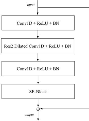
Figure 1: The SE-Res2Block of the ECAPA-TDNN architecture. The standard Conv1D layers have a kernel size of 1. The central Res2Net [14] Conv1D with scale dimension  $s = 8$  expands the temporal context through kernel size  $k$  and dilation spacing  $d$ .
