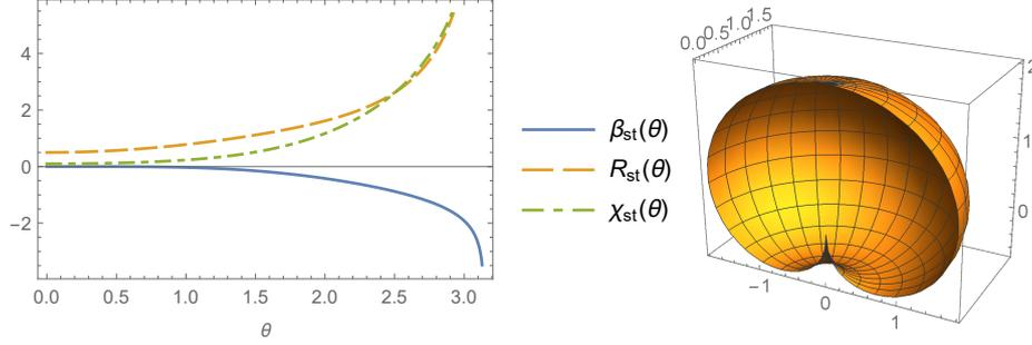
Figure 1: On the left: dependence of the stationary metric parameter  $\beta_{\text{st}}$ , the Ricci scalar  $R_{\text{st}}$  and the scalar field  $\chi_{\text{st}}$  on the extra space azimuthal angle  $\theta$ . On the right: image of the shape of two-dimensional extra space defined by the metric (13).
