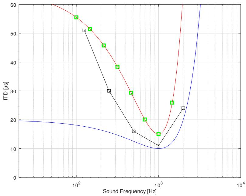
Figure 3: **The shortest JND of ITD detected in the dependence on sound frequency.** X-axis shows sound frequency in Hz in a logarithmic scale and y-axis the shortest JND of ITD in  $\mu s$ . This is a theoretical prediction based on the analytical model and basic parameter set used in simulations. As in other figures, black line is obtained by simulation and red and blue lines are respectively upper and lower bounds obtained by an analytic fit.
