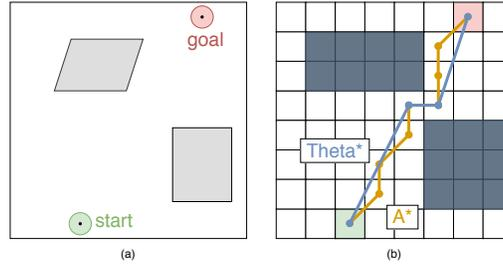
Fig. 2: Finding a path for an individual agent: a) the workspace of an agent; b) tessellation of the workspace into the grid and two paths on that grid: the one that was found by A\* (in orange) and the one that was found by THETA\* (in blue). We use THETA\* paths in this work.
