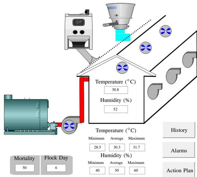
Figure 13: Layout of the implemented SCADA system.
