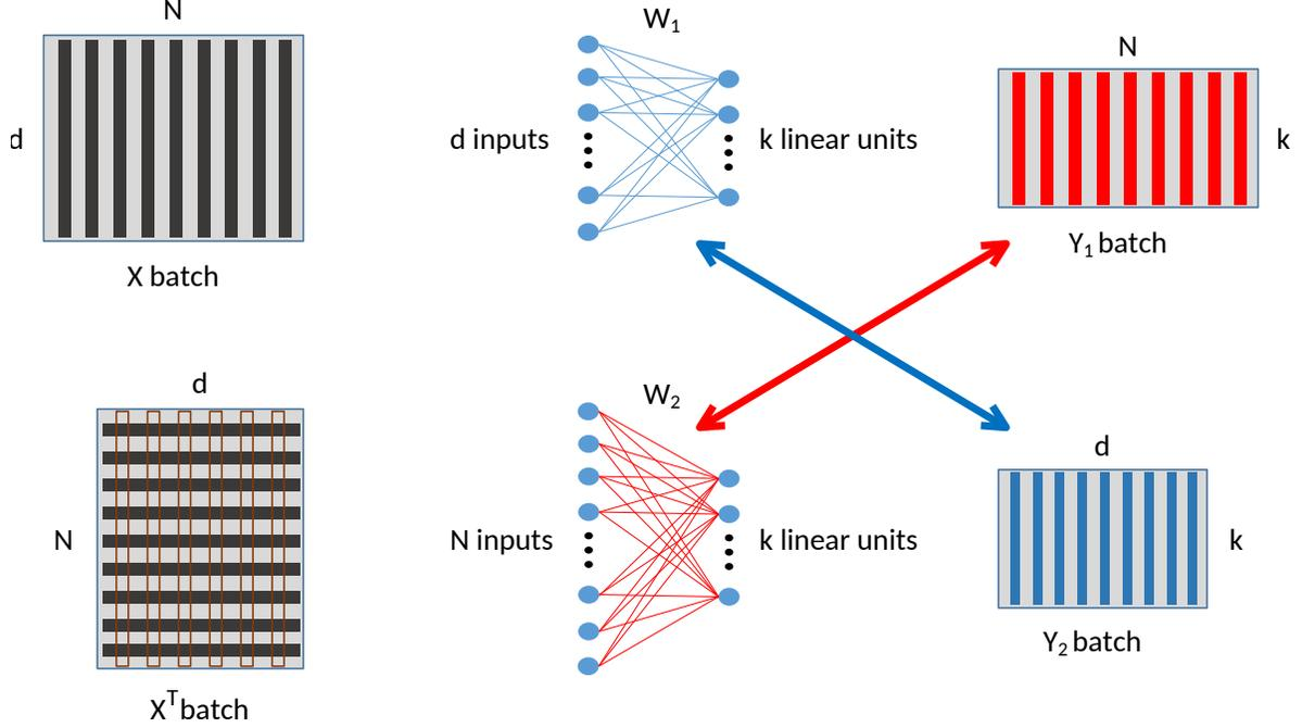
Figure 1: Dual linear single-layer neural networks.
