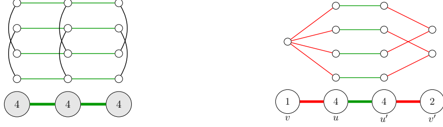
(a) A component in \Gamma_4 contains 3 splits. (b) A component in \Gamma_4 is incident to a bridge (u, v) \in \Gamma_{4,1} and a bridge (u', v') \in \Gamma_{4,2} .
