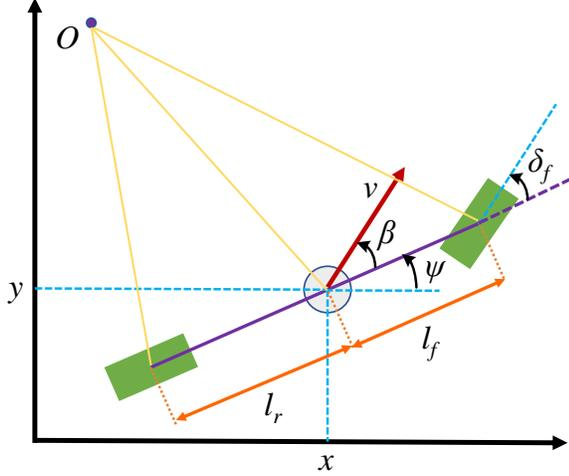
Fig. 2. Bicycle model for vehicle kinematics on highway.
