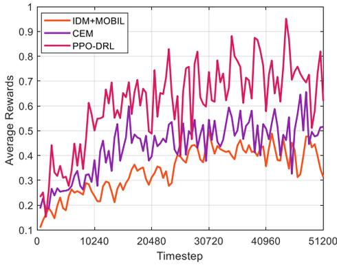
Fig. 4. Normalized average rewards in the reference model, CEM, and PPO-DRL for comparison purposes.
