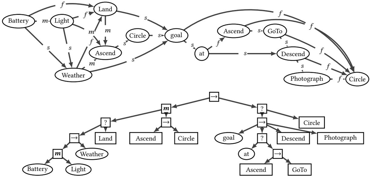
Fig. 9. (Above:) The decision structure  $Z_4$ . (Below:) A structurally equivalent 3-BT. Here we use  $\rightarrow$  and  $?$  for the operators  $*_s$  and  $*_f$  respectively, consistent with the usual notation for BTs. We use  $m$  for the operator  $*_m$ .
