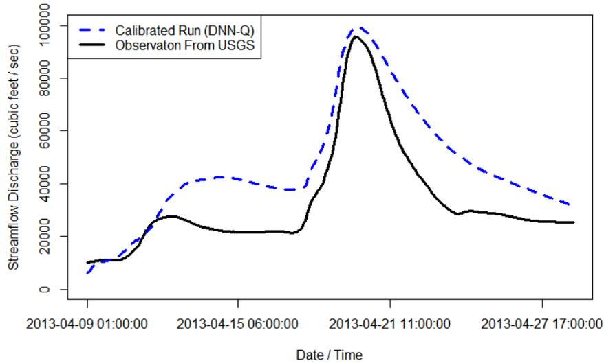
Figure 2: WRF model runs at the estimated parameter settings by DDN-Q (blue) compared to the observations from USGS (black)
