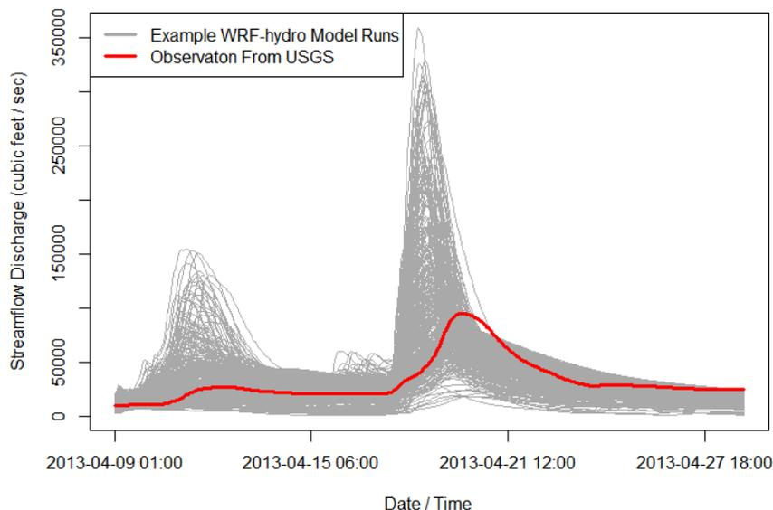
Figure 1: WRF-hydro model outputs and observational data for Iowa River at Wapello, IA (USGS ID#05465500)
