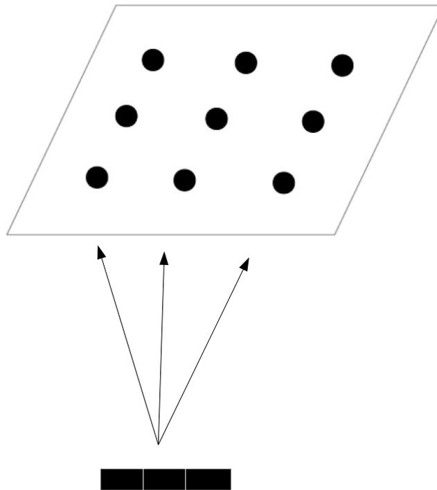
**Fig. 1.** An example of SOM. The set of rectangles stands for the input presented to the SOM (in the example the input is three-dimensional). This is presented to *all* neurons of the SOM (these are the neurons-dots-in the upper grid) in order to find the *BMU*.
