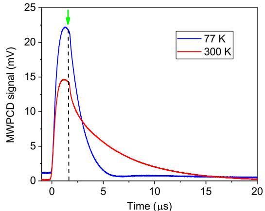
FIG. 5. *Microwave detected photoconductivity decay measurement carried out on phosphorus doped silicon. Red line shows the decay at room temperature and the blue spectrum was recorded at 77 K. The green arrow and the dashed line indicate the end of the laser pulse.*
