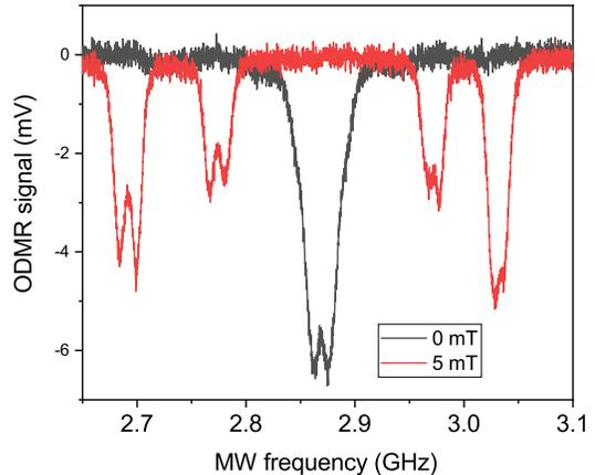
FIG. 2. *Optically detected magnetic resonance on nitrogen-vacancy centers in diamond detected at 680 nm. In zero magnetic field (black line) the resonances are degenerate while applying external magnetic field of 5 mT (red line) resolves the degeneracy.*
