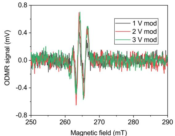
FIG. 3. *Frequency modulated and magnetic field swept ODMR measurement at 9.2 GHz on nitrogen-vacancy centers in diamond detected at 680 nm. Note that the derivative Lorentzian lineshapes are due to the frequency modulation similar to magnetic field modulation found in conventional electron spin resonance spectrometers.*
