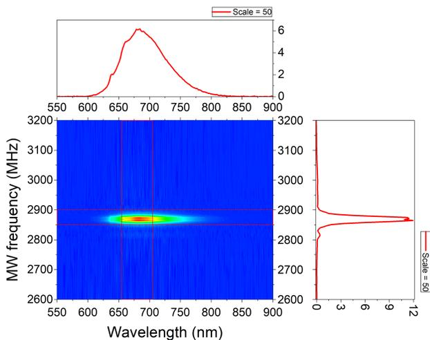
FIG. 4. *Optically detected magnetic resonance map. The upper panel is the wavelength resolved microwave frequency averaged (taken in the range 2849 – 2899 MHz) photoluminescence similar to the well-known PL spectrum of NV centers. The right panel shows a vertical profile cross section (taken in the range 655 – 705 nm), which corresponds to the microwave frequency resolved ODMR signal.*
