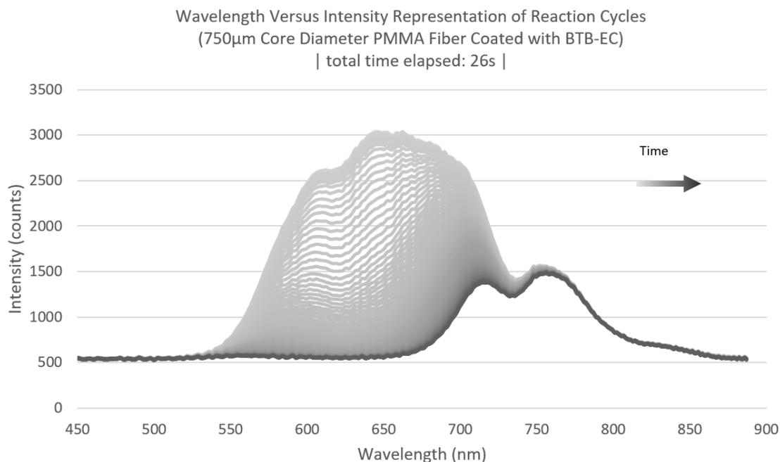
Figure 6: Transmission spectra through the FOCS, changing as the sensor is exposed to trace  $\text{NH}_3$  (darker spectral lines correspond to later times). As expected, the final state has an intensity peak throughout the 700-800nm region.
