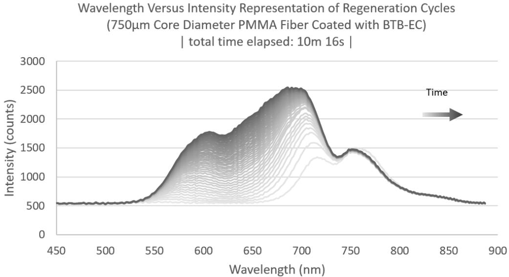
Figure 7: Transmission spectra through the FOCS, changing as the sensor regenerates from previous exposure to trace  $\text{NH}_3$  (darker spectral lines correspond to later times). The FOCS was exposed to  $\text{NH}_3$  vapor for 30s before it was purged with ambient air. The recovery process took a total of  $\sim 10$  minutes for near complete regeneration.
