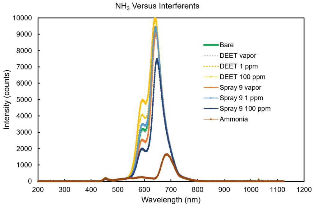
Figure 8: The effect of DEET and Spray 9 as interferents to the FOCS. We observe some response, but it is not nearly as strong as the  $\text{NH}_3$  indicating relatively good selectivity even among interferents.
