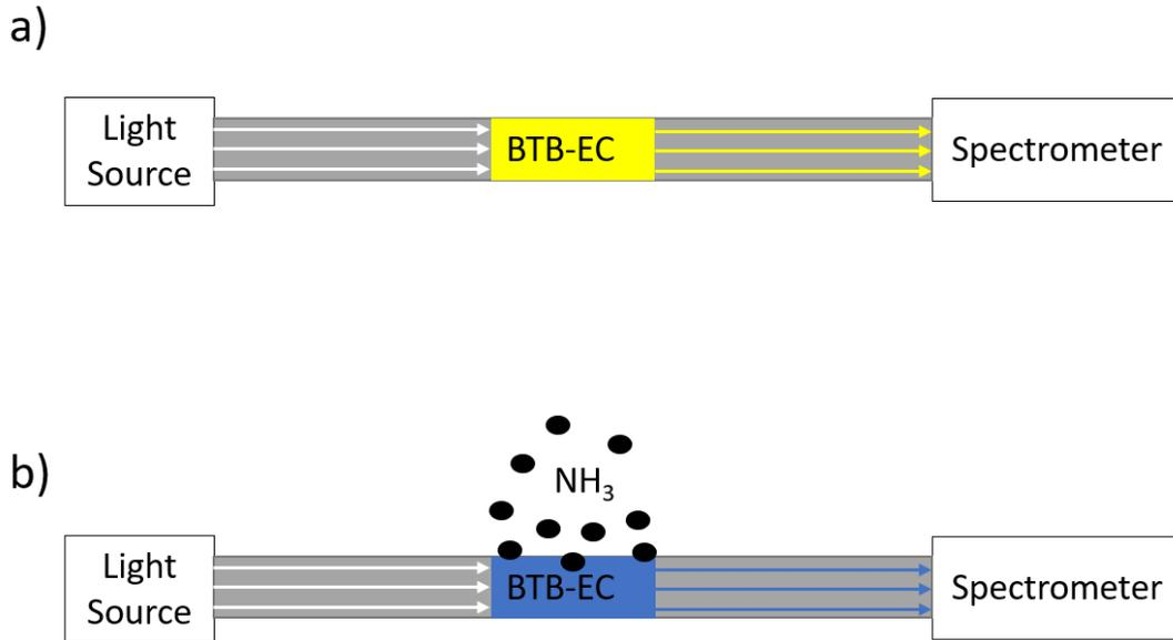
Figure 4: A schematic of the FOCS's detection process (a) before analytes reach the sensing dye, and (b) after analytes reach the sensing dye. The shift in transmission spectra detected by the spectrometer is physically realized by a physical coloration response via the BTB-EC coating.
