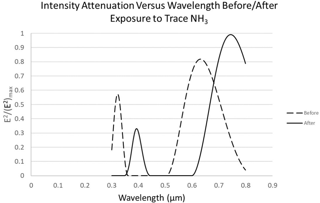
Figure 5: Graph showing the calculated strength of intensity attenuation as a function of wavelength. Before exposure to trace NH<sub>3</sub> (dotted curve), we expect strong attenuation in the blue region, giving rise to an orange/reddish color. After exposure to trace NH<sub>3</sub> (solid curve), we expect strong attenuation in the green and yellow regions, giving rise to a bluish/purplish color, as indicated by the dye's name, bromothymol blue.
