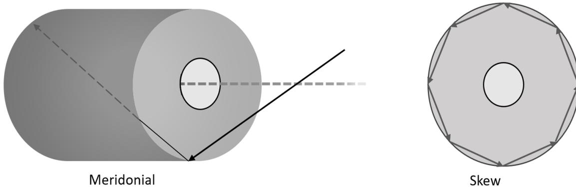
Figure 2: A visualization of meridional rays versus skew rays. The cladding material is omitted here, and pictured is just the core structure. Here, we see the two dimensional projection of the helical path of a skew ray (right). On the other hand, the schematic of the meridional ray shows the ray passing through the longitudinal axis (left).
