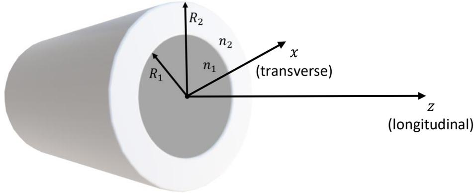
is the angle of refraction,  $n_1$  is the refractive index of the fiber core, and  $n_2$  is the refractive index of the fiber cladding.
