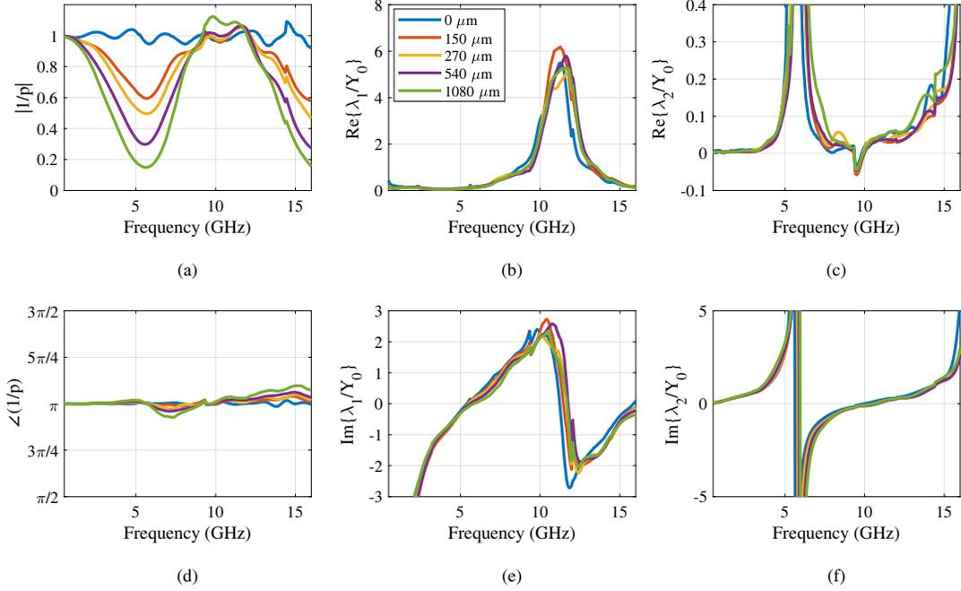
Fig. 8. Circuit parameters of the measured strip-slot unit cells for several asymmetries ( $d$  parameter) using the proposed equivalent circuit. (a) Magnitude of  $1/p$ . (b) Real part of the normalized  $\lambda_1$ . (c) Real part of the normalized  $\lambda_2$ . (d) Phase of  $1/p$ . (e) Imaginary part of the normalized  $\lambda_1$ . (f) Imaginary part of the normalized  $\lambda_2$ . ( $Z_0 = 1/Y_0 = 50 \Omega$ )
