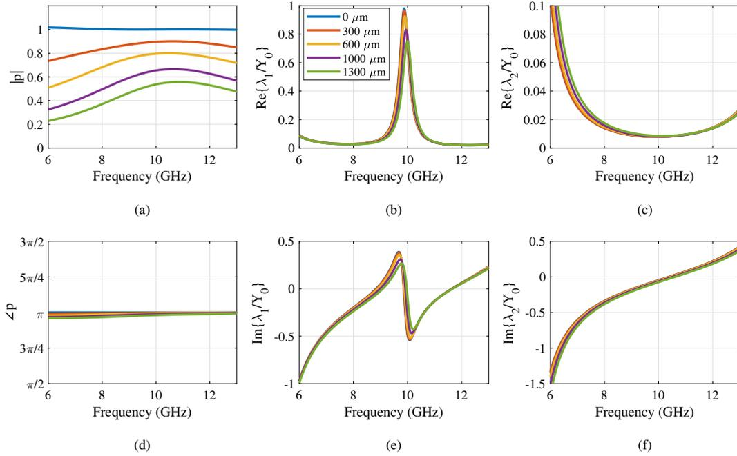
Fig. 6. Circuit parameters of the artificial SFCP unit cell for several asymmetries ( $d$  parameter) using the proposed equivalent circuit. (a) Magnitude of  $p$ . (b) Real part of the normalized  $\lambda_1$ . (c) Real part of the normalized  $\lambda_2$ . (d) Phase of  $p$ . (e) Imaginary part of the normalized  $\lambda_1$ . (f) Imaginary part of the normalized  $\lambda_2$ . ( $Z_0 = 1/Y_0 = 50 \Omega$ )
