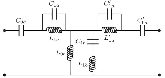
Fig. 3. Artificial CRLH transmission line unit cell.  $C_{0a} = 7.45$  pF,  $L_{1a} = 3.09$  nH,  $C_{1a} = 1.86$  pF,  $C'_{0a} = 5.59$  pF,  $L'_{1a} = 2.55$  nH,  $C'_{1a} = 2.05$  pF,  $L_{0b} = 15.38$  nH,  $L_{1b} = 6.21$  nH,  $C_{1b} = 1.23$  pF
