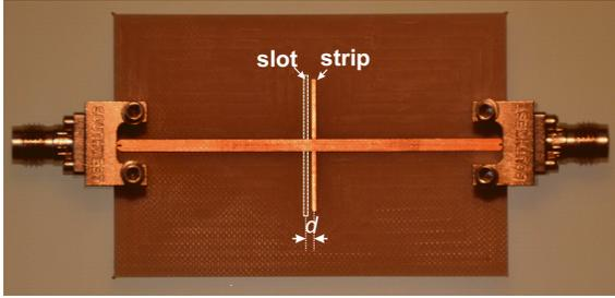
Fig. 7. Backlit photograph of a prototype of the complementary strip-slot with certain misalignment  $d$ .
