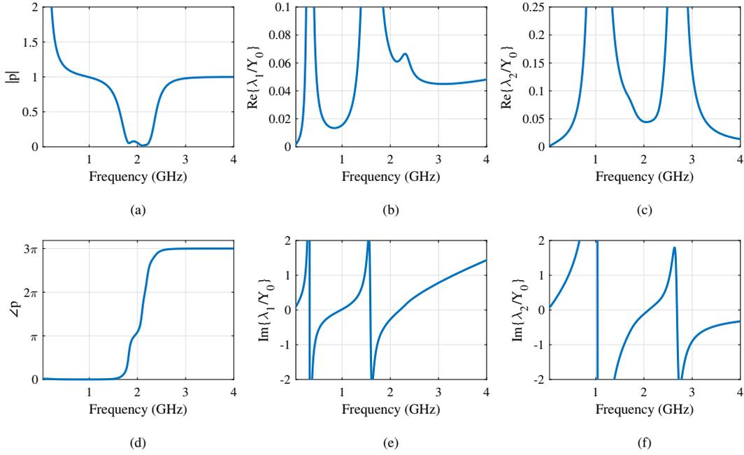
Fig. 4. Circuit parameters of the artificial CRLH transmission line unit cell using the proposed equivalent circuit. (a) Magnitude of  $p$ . (b) Real part of the normalized  $\lambda_1$ . (c) Real part of the normalized  $\lambda_2$ . (d) Phase of  $p$ . (e) Imaginary part of the normalized  $\lambda_1$ . (f) Imaginary part of the normalized  $\lambda_2$ . ( $Z_0 = 1/Y_0 = 50 \Omega$ )
