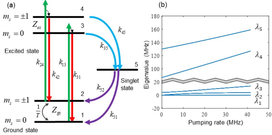
Figure 1 (a) Energy level structure of the NV center. (b) the change in five eigenvalues with respect to the optical pumping rate ( $\Gamma$ ).
