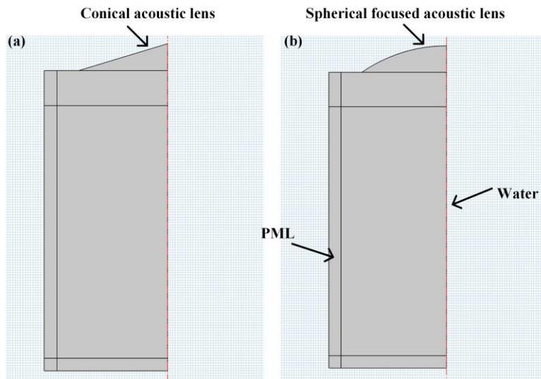
Figure 2. Simulation using COMSOL. (a) Conical acoustic lens. (b) Spherical focused acoustic lens.
