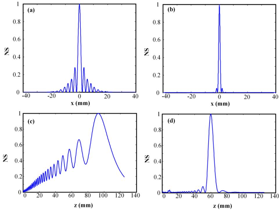
Figure 4. Quantitatively measure the performance of the conical acoustic lens. (a) and (c) are the sound intensity distributions of conical acoustic lens and spherical acoustic lens on the central axis, respectively. (b) and (d) The sound field intensity of the conical acoustic and spherical acoustic lens in the lateral direction, respectively. NS, normalize strength.
