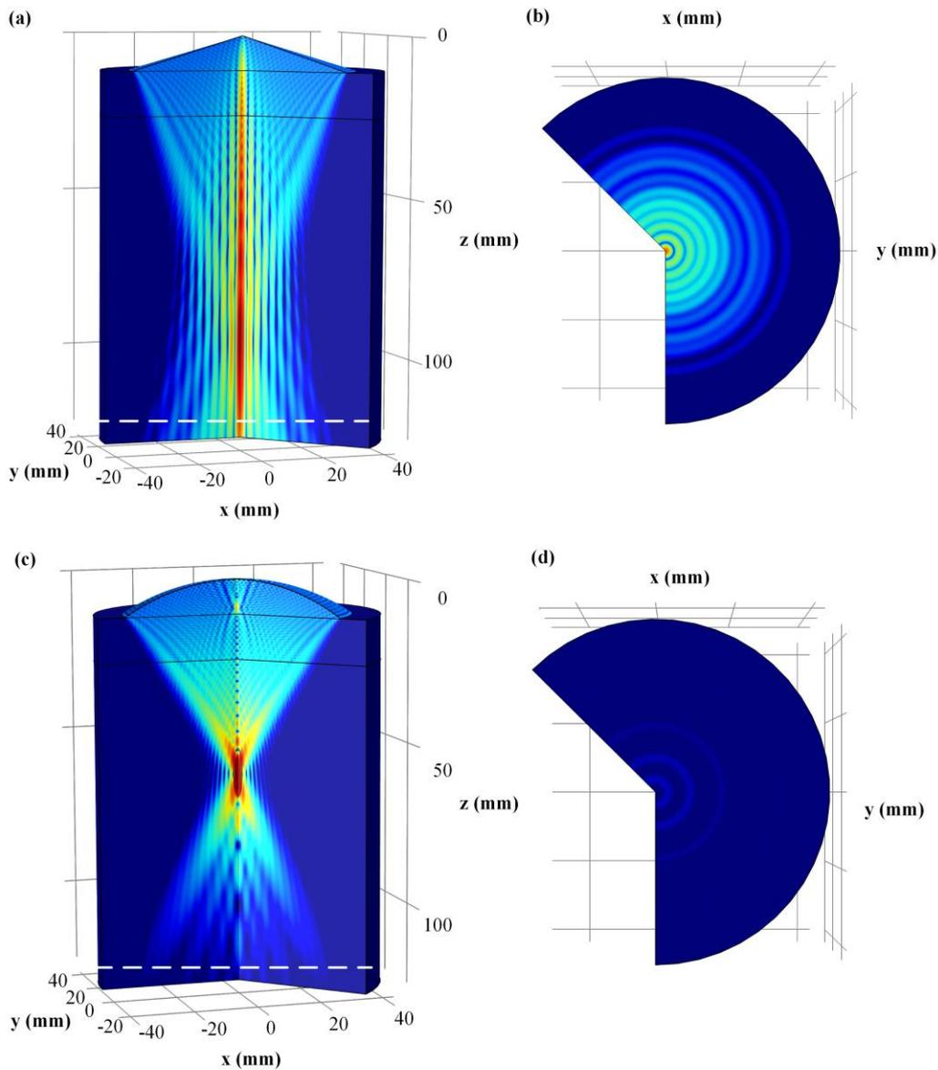
Figure 3. Simulation. (a) The sound field of the conical acoustic lens. (b) The lateral distribution of the sound field indicated by the white dashed line in (a). (c) The sound field of the spherical acoustic lens. (d) The lateral distribution of the sound field indicated by the white dashed line in (c).
