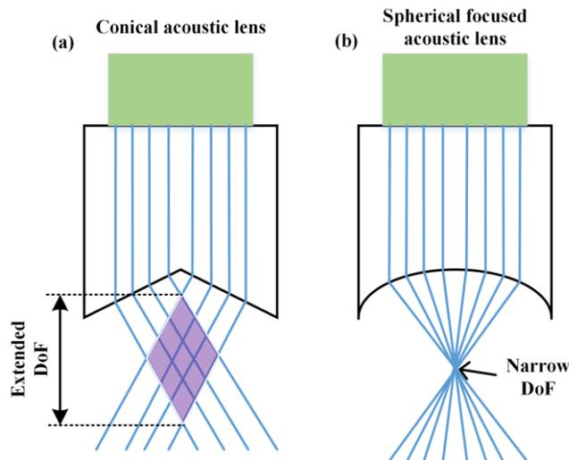
Figure 1. Design of conical acoustic lens. (a) Conical acoustic lens. (b) Spherical focused acoustic lens.
