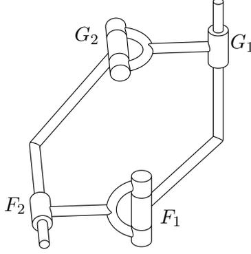
Figure 4: An RCRC-mechanism constructed from a quadratic polynomial.
