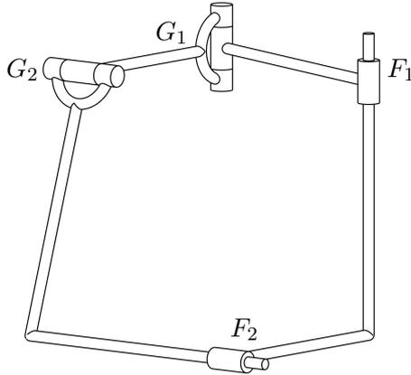
Figure 3: An RRCC-mechanism to perform a Bennett motion.
