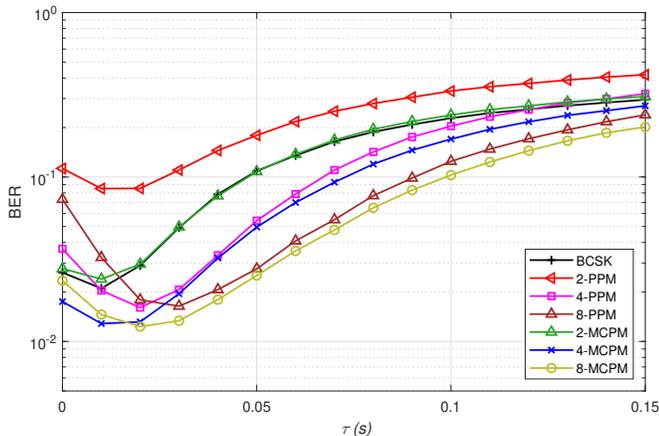
Fig. 13. BER vs.  $\tau$  curves for MCPM and competing schemes.  $M = 50$  molecules,  $t_b = 0.30$  s,  $r_0 = 10 \mu\text{m}$ ,  $r_r = 5 \mu\text{m}$ ,  $D = 79.4 \mu\text{m}^2 \text{s}^{-1}$ ,  $t_{\text{total}} = 48t_b$ .
