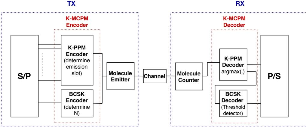
Fig. 4. Overall transmission and reception model of an MCD system utilizing  $\mathcal{K}$ -MCPM and the TPCD.
