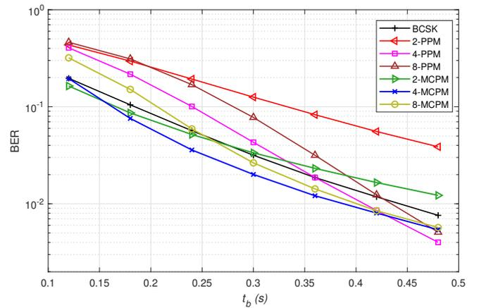
Fig. 12. BER vs.  $t_b$  curves for MCPM and competing schemes.  $M = 50$  molecules,  $r_0 = 10 \mu\text{m}$ ,  $r_r = 5 \mu\text{m}$ ,  $D = 79.4 \mu\text{m}^2 \text{s}^{-1}$ , and  $t_{\text{total}} = 30$  s.
