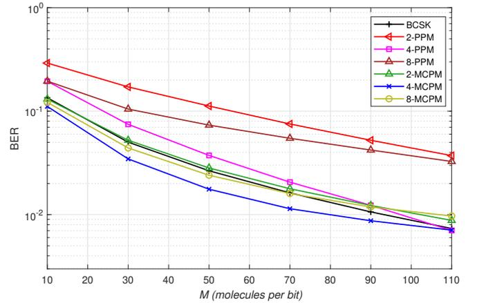
Fig. 11. BER vs.  $M$  curves for MCPM and competing schemes.  $t_b = 0.30$  s,  $r_0 = 10 \mu\text{m}$ ,  $r_r = 5 \mu\text{m}$ ,  $D = 79.4 \mu\text{m}^2 \text{s}^{-1}$ , and  $t_{\text{total}} = 48t_b$ .
