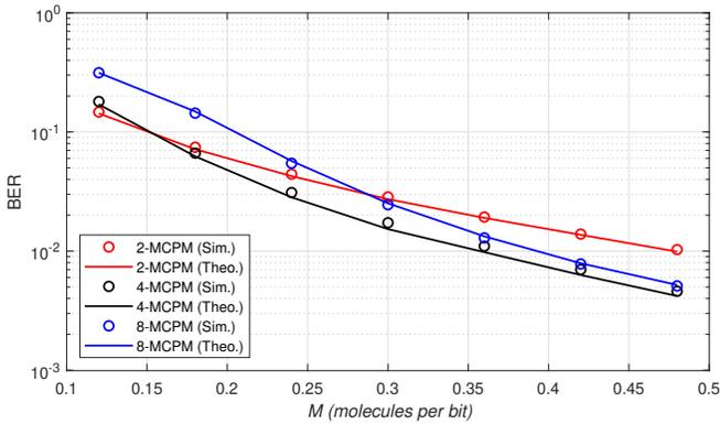
Fig. 6. BER vs.  $t_b$  curves.  $M = 50$  molecules,  $r_0 = 10\mu\text{m}$ ,  $r_r = 5\mu\text{m}$ ,  $D = 79.4 \frac{\mu\text{m}^2}{\text{s}}$ , and  $t_{\text{total}} = 12t_b$ .  $(\alpha, \gamma)$  pairs optimized through exhaustive search.
