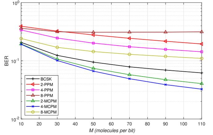
Fig. 10. BER vs.  $M$  curves for MCPM and competing schemes.  $t_b = 0.18$  s,  $r_0 = 10 \mu\text{m}$ ,  $r_r = 5 \mu\text{m}$ ,  $D = 79.4 \mu\text{m}^2 \text{s}^{-1}$ , and  $t_{\text{total}} = 48t_b$ .
