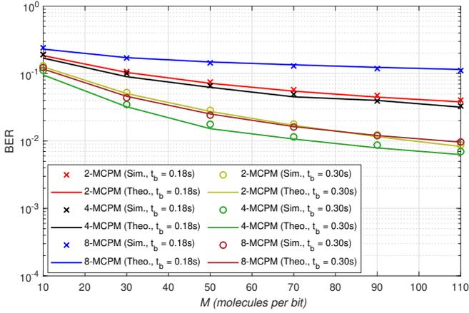
Fig. 5. BER vs.  $M$  curves.  $t_b = 0.18$  and  $0.30$ s,  $r_0 = 10\mu\text{m}$ ,  $r_r = 5\mu\text{m}$ ,  $D = 79.4 \frac{\mu\text{m}^2}{\text{s}}$ , and  $t_{\text{total}} = 12t_b$ .  $(\alpha, \gamma)$  pairs optimized through exhaustive search.
