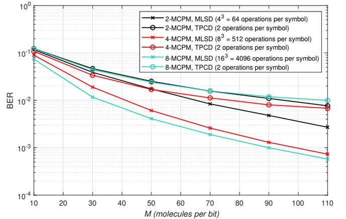
Fig. 3. BER vs.  $M$  curves for MCPM using MLSD and TPCD.  $t_b = 0.30$  s,  $r_0 = 10$   $\mu\text{m}$ ,  $r_r = 5$   $\mu\text{m}$ ,  $D = 79.4$   $\mu\text{m}^2 \text{s}^{-1}$ ,  $L_s = 3$ .  $\alpha$  and  $\gamma$  numerically optimized.
