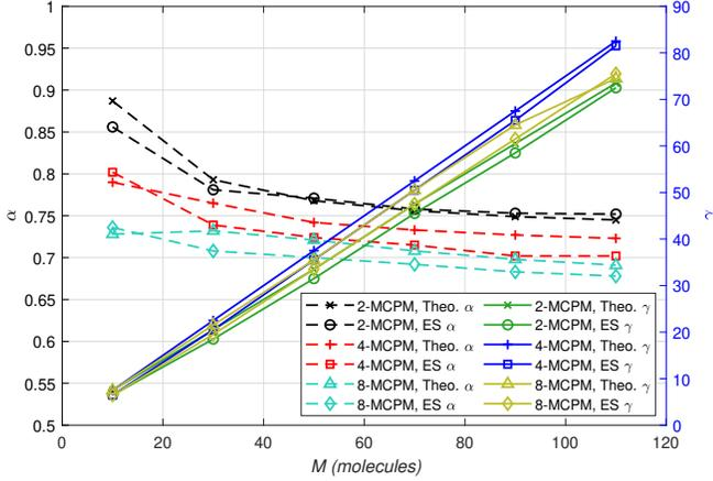
Fig. 7.  $\alpha$  and  $\gamma$  vs.  $M$  for MCPM, using theoretical and simulated values.  $t_b = 0.30$  s,  $r_0 = 10$   $\mu\text{m}$ ,  $r_r = 5$   $\mu\text{m}$ ,  $D = 79.4$   $\mu\text{m}^2 \text{s}^{-1}$ , and  $t_{\text{total}} = 48t_b$ .
