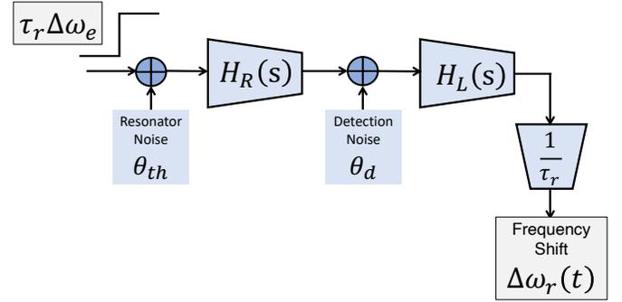
Fig. 7. Phase-domain model for FF scheme
