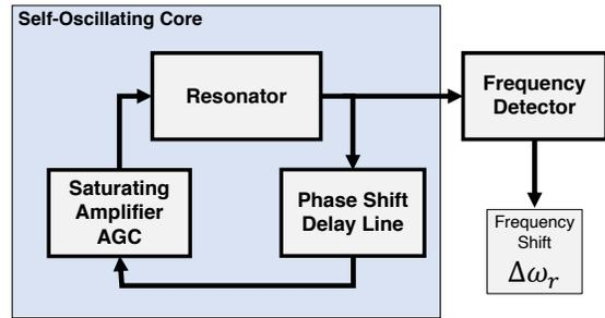
Fig. 3. Self-sustained oscillator (figure based on [12, Fig. 1])
