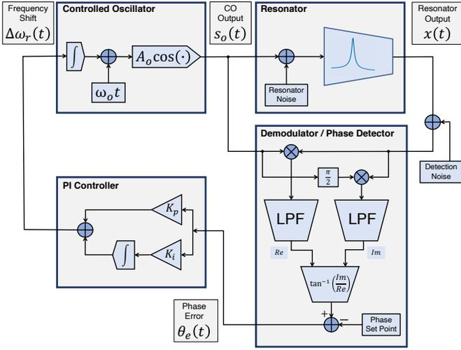
Fig. 5. Frequency-locked loop (FLL) (figure based on [12, Fig. 2])
