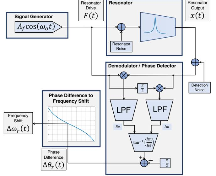
Fig. 4. Feedback-free (FF) scheme (figure based on [12, Fig. 2])
