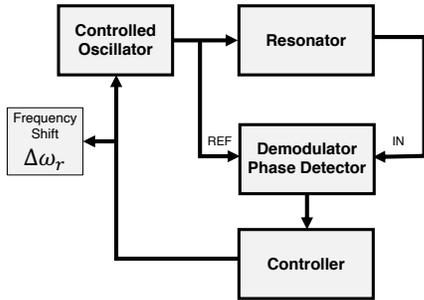
Fig. 2. Frequency-locked loop (figure based on [12, Fig. 1])
