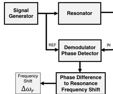
Fig. 1. Feedback-free resonator tracking (figure based on [12, Fig. 1])
