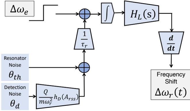
Fig. 9. Phase-domain model for SSO
