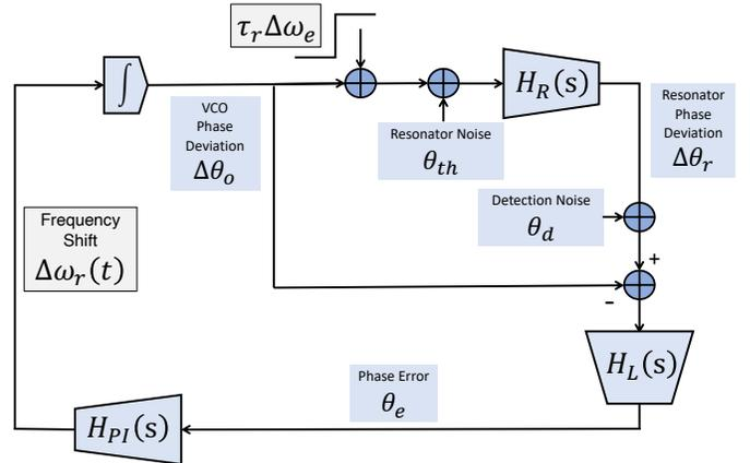
Fig. 8. Phase-domain model for FLL (figure based on [12, Fig. 3])
