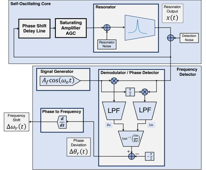
Fig. 6. Self-sustained oscillator (SSO) (figure based on [12, Fig. 2])
