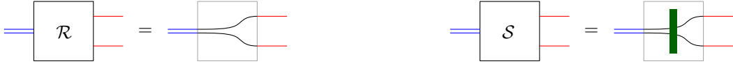
FIGURE 5. The diagrams for the realignment tester \mathcal{R} and the SIC POVM tester \mathcal{S} . The (green) solid rectangle in the diagram for \mathcal{S} is the symmetrization operation in Penrose’s graphical formalism. The two blue output wires are treated as a single vector space \mathbb{C}^n = \mathbb{C}^{d^2} .
