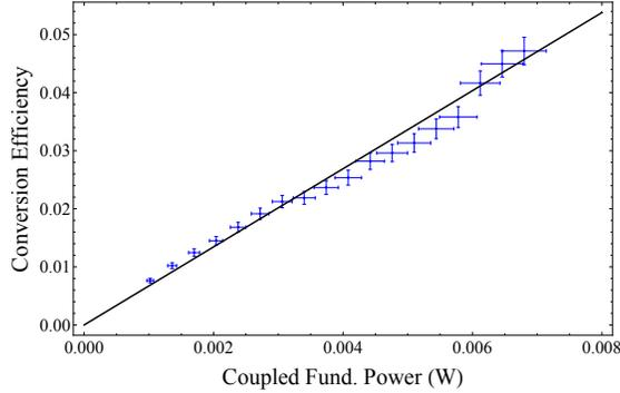
Figure 3: SH Power exiting the waveguide resonator as the fundamental power entering the resonator is varied. The black line shows the predicted SHG with a nonlinear efficiency of  $11\% / (\text{W}\cdot\text{cm})^2$  using the presented theory, while the blue lines indicates the measured SH powers with associated error bars.
