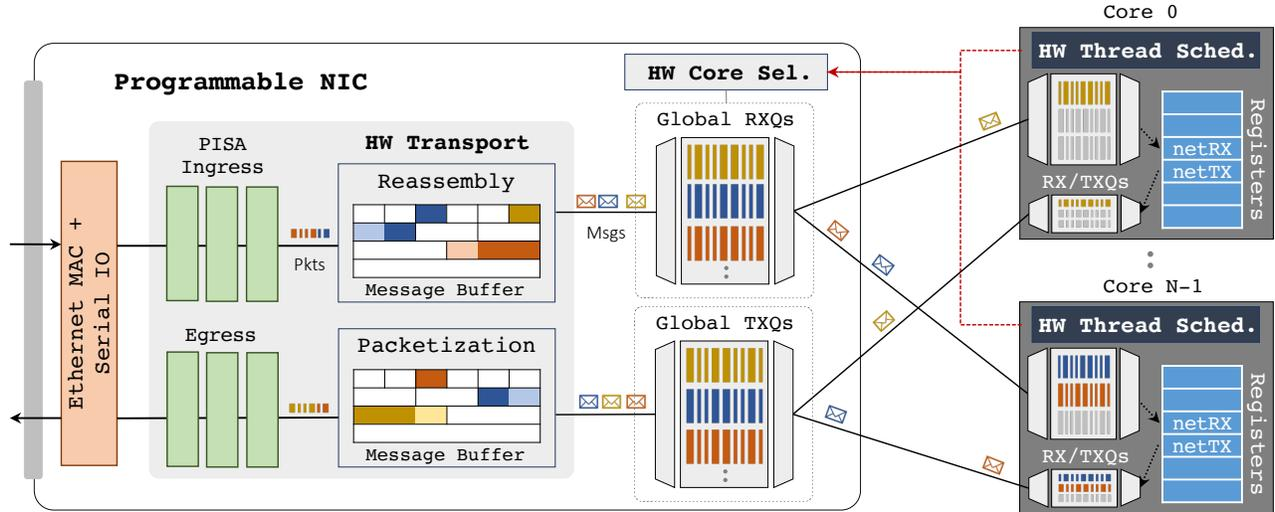
**Figure 1: The nanoPU design.** The NIC includes ingress and egress PISA pipelines as well as a hardware-terminated transport and a core selector with global RX queues; each CPU core is augmented with a hardware thread scheduler and local RX/TX queues connected directly to the register file.
