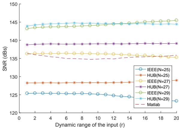
**Fig. 8** Precision of different Givens rotation units when varying  $r$  (dynamic range of the input)
