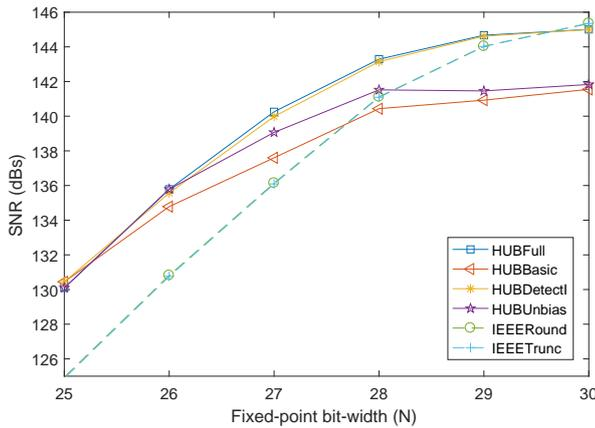
**Fig. 10** Precision of different approaches when varying  $N$  (internal significand bit-width)
