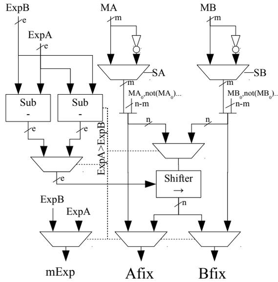
**Fig. 5** FP to fixed-point HUB converter
