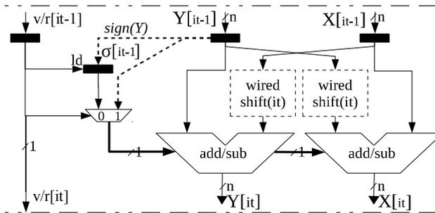
Fig. 3 Pipelined stage for fixed-point Givens rotation unit
