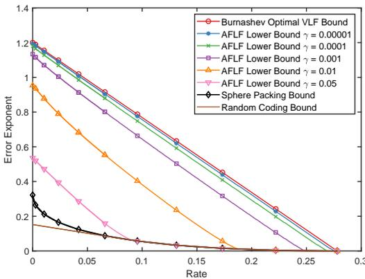
Fig. 4. Figure shows the error exponents achieved by AFLF codes when  $K \geq K^* = 7$  for values of  $\gamma$  approaching zero. The AFLF bounds are compared with the Burnashev's optimal VLF exponent along with upper bound and lower bound on FLF codes i.e., sphere packing bound and random coding bound for a BSC with cross-over probability  $p = 0.2$ .
