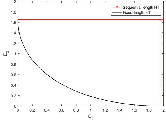
Fig. 2. Figure shows the optimal error exponents of fixed-length hypothesis test and sequential hypothesis test for Bernoulli samples with parameters given by  $p_1 = 0.9$  under  $H_1$  and  $p_2 = 0.2$  under  $H_2$ .
