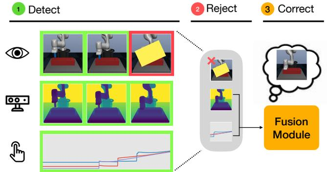
Fig. 1: We propose Crossmodal Compensation Model that can (1) **detect** when a sensor input is corrupted, which in this case is the image data, (2) **reject** the corrupted image as input to our policy, and (3) **correct** for the rejected image by compensating the missing image information with the remaining force and depth information in the fusion module.
