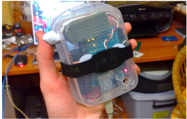
Figure 3: Our networked heartbeat sensor in action.
