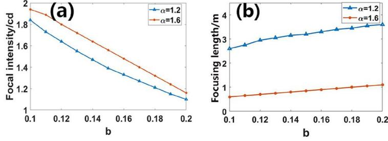
Fig. 9. (color online) (a) The focal intensity and (b) focusing length versus distribution parameter  $b$  in input (3), for the autofocusing split vortex pair, at two fixed values of LI,  $\alpha = 1.2$  and  $\alpha = 1.6$ .
