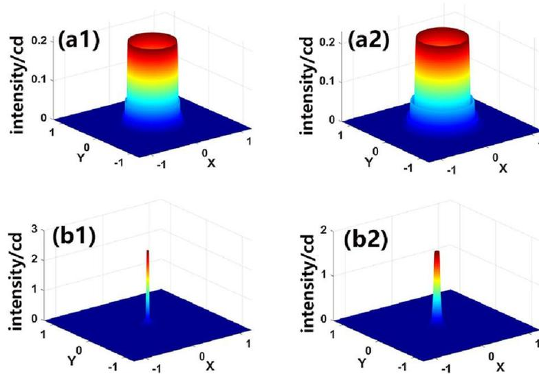
Fig. 4. (color online) Intensity distributions in the input and in the tightest autofocused state for  $b = 0.06$  (a1,b1) and  $b = 0.1$  (a2,b2). Other parameters are  $m = 1, \alpha = 1.4$ . Note the difference in the scales of the vertical axes between the top and bottom panels.
