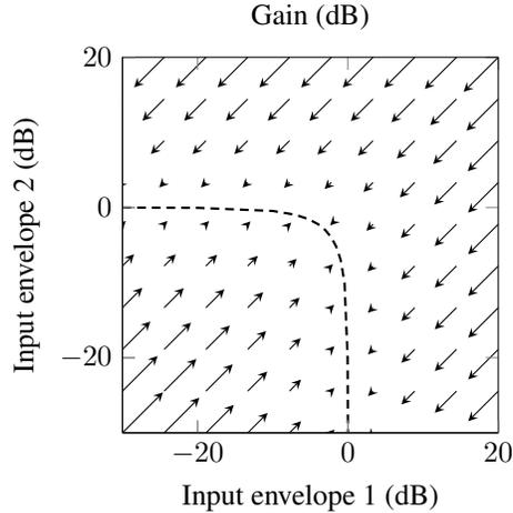
Figure 4: Gain applied to a mixture signal as a function of the signal envelopes  $v_{s_1}[t, b]$  and  $v_{s_2}[t, b]$  for  $\mathcal{C}_b(v) = v^{1/3}$  under Assumption 1. The length of the arrows is proportional to the power gain  $g^2[t, b]$  in dB and the dashed curve shows the equilibrium mixture level  $\mathcal{C}_b(v_{s_1} + v_{s_2}) = v_{s_1} + v_{s_2}$ . The axes are scaled so that this equilibrium level is 0 dB.
