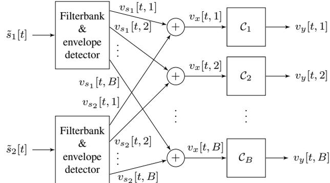
Figure 3: A simplified model separates the effects of the filterbank and envelope detector from those of the compression functions  $C_b$ . The former is assumed to act independently across component signals, while the latter act independently across time and channels.
