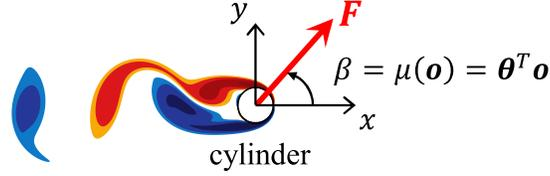
FIG. 3. Configuration of the cylinder forcing problem. Reinforcement learning optimizes the policy  $\beta$ , the direction of forcing, to maximize the average speed of the cylinder  $\langle V_x \rangle$ .
