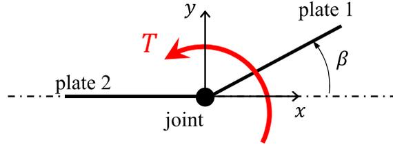
FIG. 6. Configuration of the swimming problem. The hinge is driven by the external torque  $T$  acting on the plate 1. Reinforcement learning optimizes  $T$  to maximize the average speed of the hinge  $-\langle \dot{x}_h \rangle$ .
