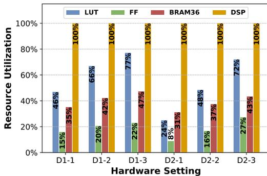
Fig. 4. **FPGA resource utilization with different devices and settings.** In the three designs for each of the two devices, the DSP utilization is maintained at 100% and the LUT utilization is raised to 70%–80% with FF and BRAM resources.
