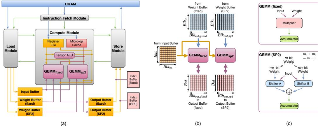
Fig. 3. **Hardware architecture of convolution for MSQ number system.** (a) Overall framework with  $GEMM_{fixed}$  core for fixed-point operations and  $GEMM_{fixed}$  core for SP2 operations; (b) Dataflow in heterogeneous GEMM cores; and (c) Computations in heterogeneous GEMM cores.
