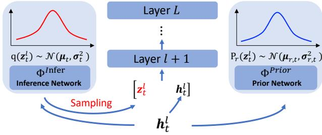
Fig. 2. An example Variational TDNN. Note that the output vector of  $l$ -th layer  $\mathbf{h}_t^l$  is used as the input of the inference network  $\Phi^{Infer}$  and prior network  $\Phi^{Prior}$  to calculate the mean and variance of the latent variable variational and prior distributions respectively. Then we concatenate the latent variable  $\mathbf{z}_t^l$  sampled from the inference network  $\Phi^{Infer}$  with  $\mathbf{h}_t^l$  as the input of the  $(l+1)$ -th layer.
