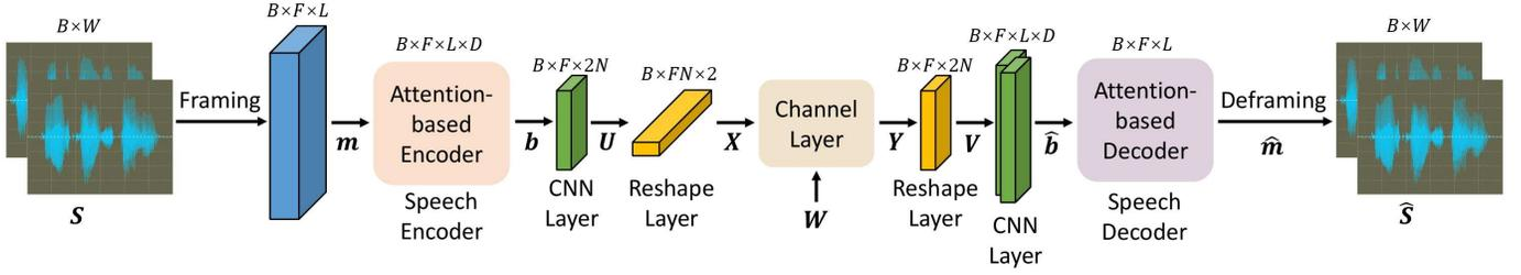
Fig. 2: The proposed system architecture for semantic communication system for speech signals.
