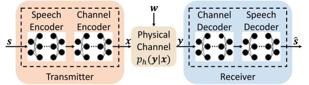
Fig. 1: The model structure of DL-enabled semantic communication system for speech signals.
