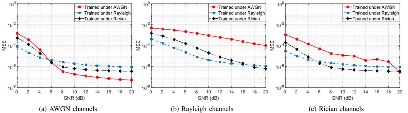
Fig. 4: MSE loss tested for (a) AWGN, (b) Rayleigh, and (c) Rician channels with the models trained under various channels.
