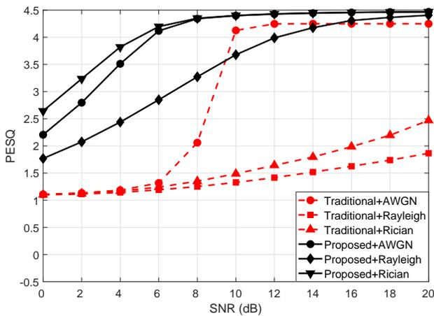
Fig. 6: PESQ score versus SNR for the traditional speech communication systems with 8-bits A-law PCM coding with Turbo codes in 64-QAM and DeepSC-S under the AWGN channels, the Rayleigh channels, and the Rician channels.
