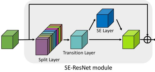
Fig. 3: SE-ResNet module for constructing the *speech encoder* and the *speech decoder*.
